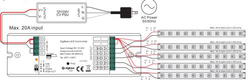
Note: please make sure the dial switches are at position for DIM mode as shown in above diagram.
