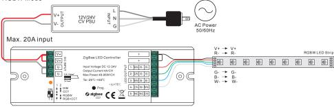
Note: please make sure the dial switches are at position for RGBW mode as shown in above diagram.
