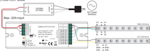
Note: please make sure the dial switches are at position for RGB+CCT mode as shown in above diagram.
