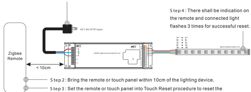
Step 4: There shall be indication on the remote and connected light flashes 3 times for successful reset.
