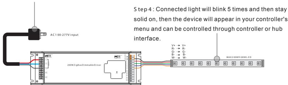
Step 4: Connected light will blink 5 times and then stay solid on, then the device will appear in your controller's menu and can be controlled through controller or hub interface.
