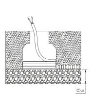
Install the sleeves on the ground,the top side should on the same level with the ground surface,cable need to go through the sleeve.
