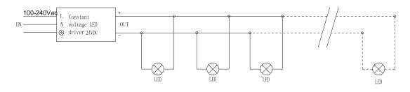
Explanations:the transmiss circuit of the whole group depends on the circuit of junction boxes. the max. current depends on the max. load of power cable between the junction boxer,but it is not related to the max. load current of power cable of the fitting. The outer diameter of cable between the junction boxes is limited by the max. outer diameter of speedy plug,the max. allowed outer diameter is 10mm.
